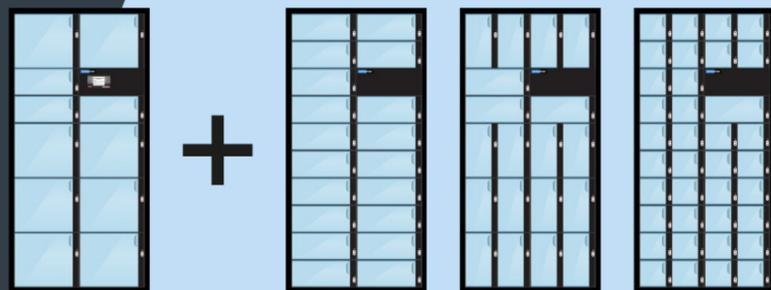
Install up to 3 SupplyVend Auxiliary units to one SupplyVend Main unit. Auxiliaries can be all the same or mix of any available door configurations.
